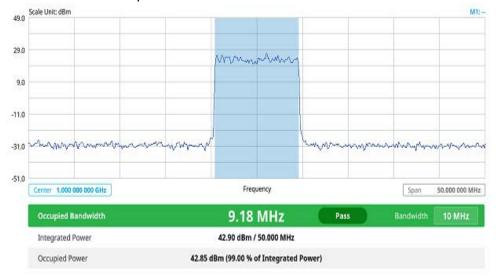
The Occupied Bandwidth measurement shows both of power across the band and power bandwidth in a user specified percentage to determine the amount of spectrum
