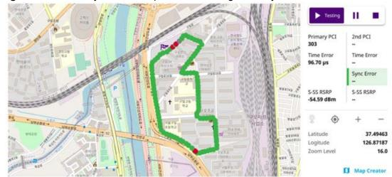
Figure 137 Online sync route map with 5G NR Signal Analyzer
