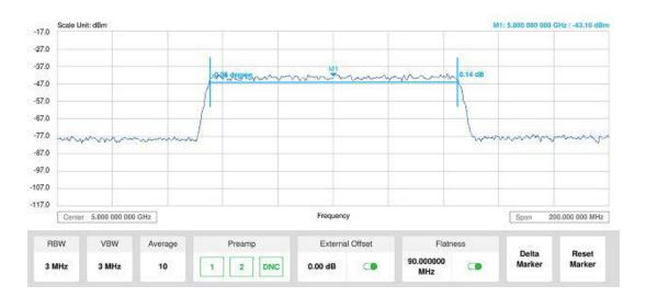
Figure 87 PIM detection — single carrier
