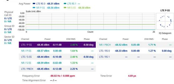
Figure 192 5G DSS OTA Control Channel measurement
