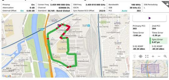
Figure 132 Sync route map with 5G NR Signal Analyzer
