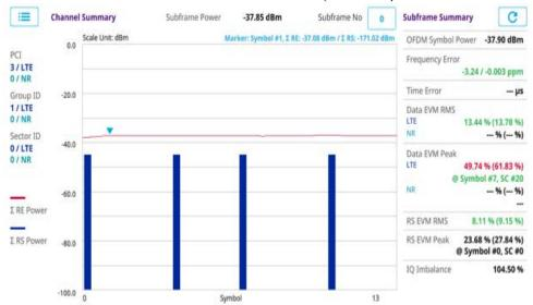
Figure 205 5G DSS DSS subframe measurement (bar chart)
