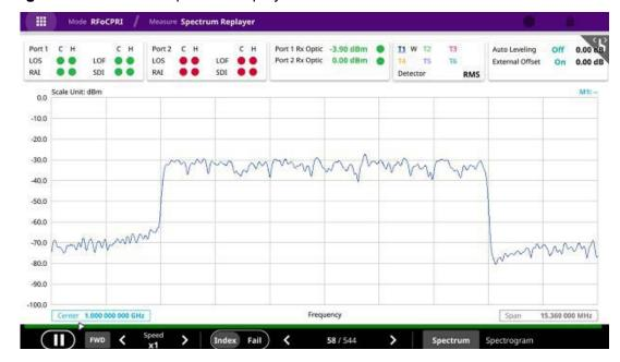
Figure 59 RFoCPRI spectrum replay
