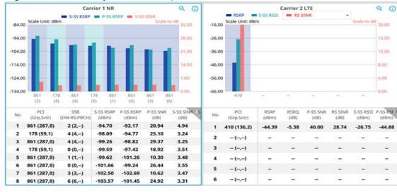
Figure 171 NSA Analyzer with sweep normal measurement
