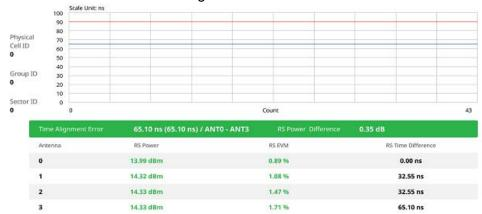
Figure 266 LTE/LTE-A TDD time alignment error measurement
