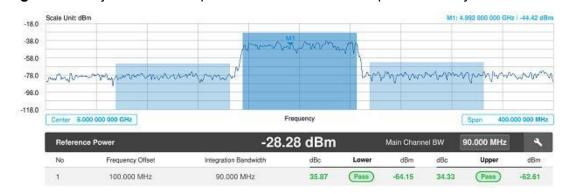
Figure 20 Adjacent channel power measurement with Spectrum Analyzer
