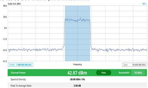
Figure 183 5G DSS channel power measurement
