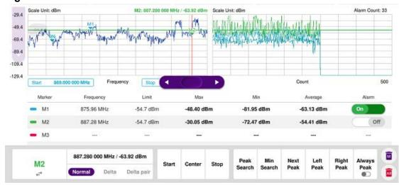
Figure 81 Interference measurement in RSSI
