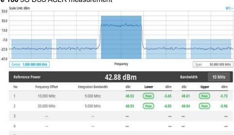
Figure 186 5G DSS ACLR measurement
