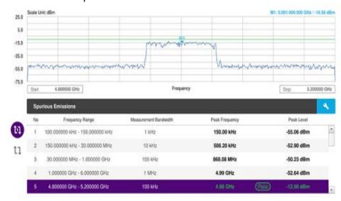
Figure 188 5G DSS spurious emissions measurement
