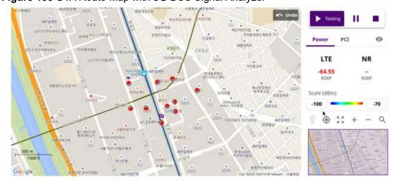
Figure 193 OTA Route Map with 5G DSS Signal Analyzer
