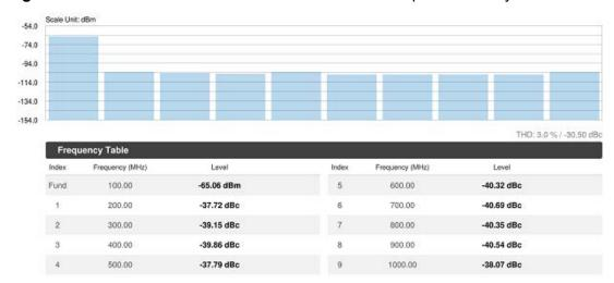
Figure 24 Total harmonic distortion measurement with spectrum analyzer
