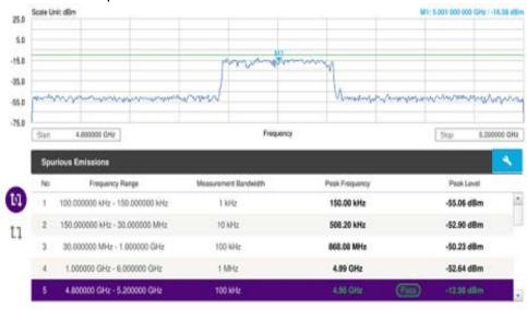
Figure 111 5G NR spurious emissions measurement
