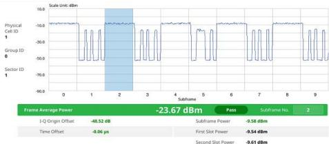
Figure 238 LTE/LTE-A FDD Power vs Time (Frame) measurement
