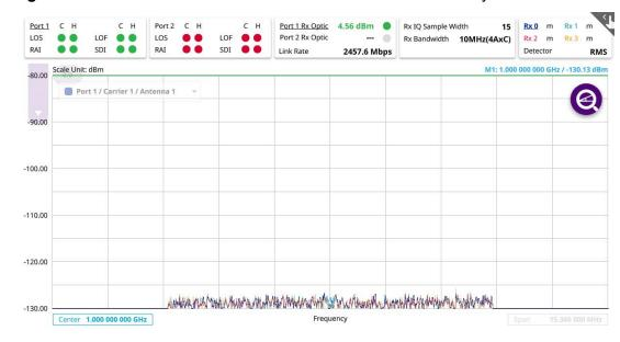
Figure 49 PIM check chart view with RFoCPRI Interference Analyzer
