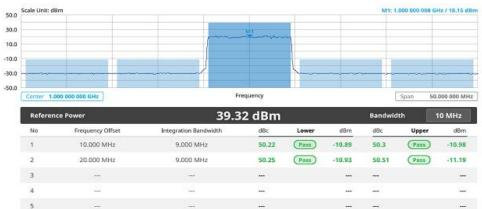
Figure 215 LTE/LTE-A FDD ACLR measurement
