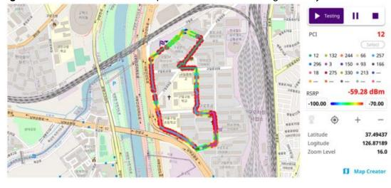
Figure 239 Online OTA Route Map with LTE/LTE-A FDD Signal Analyzer
