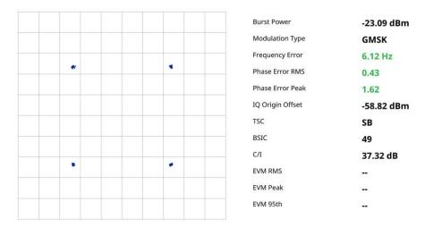
Figure 288 Constellation measurement (on) in GSM
