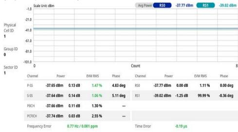
Figure 254 LTE/LTE-A TDD OTA control channel measurement
