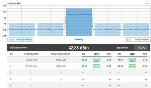
Figure 246 LTE/LTE-A TDD ACLR measurement
